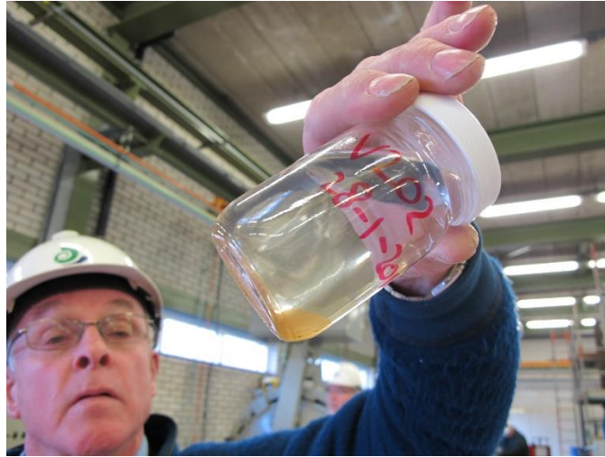
Figure 5: Clean condensate above water as sampled from the Twister Hydrate Separator
